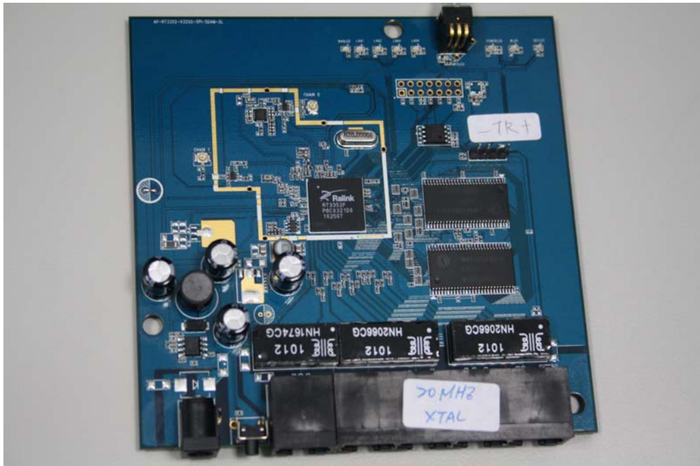
Figure 4 The RT3352 Demo Board
